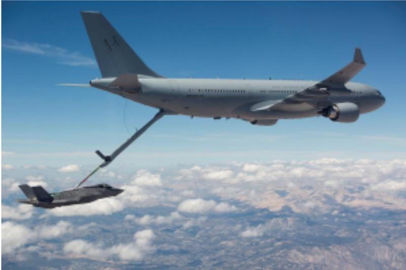
The Royal Australian Air Force (RAAF) has completed the first fuel transfer with the air refuelling boom from a RAAF KC-30A Multi-Role Tanker Transport (MRTT) to a US Air Force (USAF) F-35A Joint Strike Fighter at Edwards Air Force Base in California. A total of 59 contacts were conducted of which five contacts transferred 43,200 pounds of fuel during the four hour sortie.
